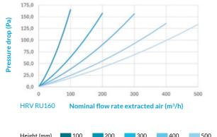
Based on test conditions following NEN-EN 308:2022 (Environmental conditions: temp. 5°C, humidity 70%; inside conditions: 25°C, humidity 25%) Calculate your specific conditions with our CORE Online Calculator.
