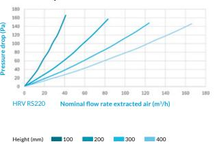
Based on test conditions following NEN-EN 308:2022 (Environmental conditions: temp. 5°C, humidity 70%; inside conditions: 25°C, humidity 25%) Calculate your specific conditions with our CORE Online Calculator.
