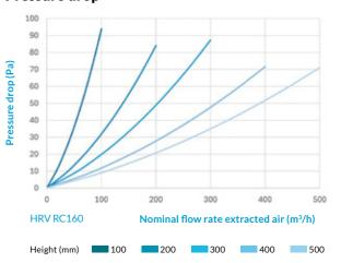
Based on test conditions following NEN-EN 308:2022 (Environmental conditions: temp. 5°C, humidity 70%; inside conditions: 25°C, humidity 25%) Calculate your specific conditions with our CORE Online Calculator.
