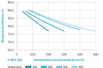
Based on test conditions following NEN-EN 308:2022 (intake air: temp. 5°C, humidity 70%; extracted air: 25°C, humidity 50%) Calculate your specific conditions with our Core Online Calculator
