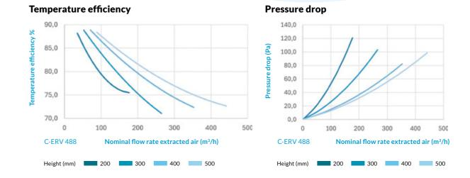
Based on test conditions following NEN-EN 308:2022 (intake air: temp. 5°C, humidity 70%; extracted air: 25°C, humidity 50%) Calculate your specific conditions with our CORE Online Calculator.
