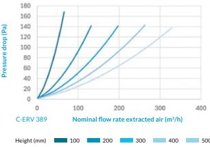
Based on test conditions following NEN-EN 308:2022 (intake air: temp. 5 °C, humidity 70 %; extracted air: 25 °C, humidity 50 %) Calculate your specific conditions with our CORE Online Calculator.
