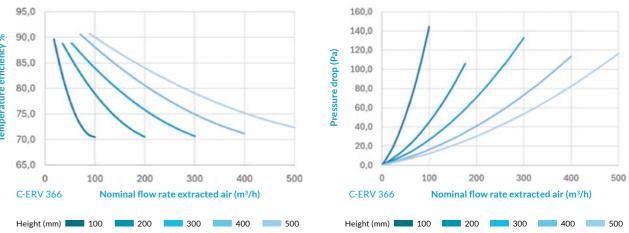
Based on test conditions following NEN-EN 308:2022 (intake air: temp. 5°C, humidity 70%; extracted air: 25°C, humidity 50%) Calculate your specific conditions with our Core Online Calculator.
