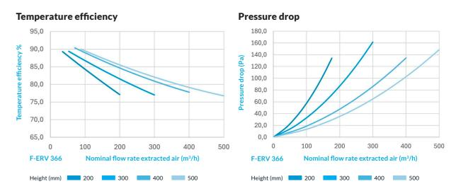
Based on test conditions following NEN-EN 308:2022 (intake air: temp. 5°C, humidity 70%; extracted air: 25°C, humidity 50%) Calculate your specific conditions with our Core Online Calculator
