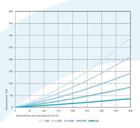
\*Based on test conditions following DIN EN 308:1997-06 (Environmental conditions: intake air temp. 5°C, humidity 70%; extracted air: 25°C, humidity 50%)
