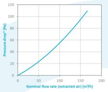
\*Based on a CORE height of 400 mm, test conditions following DIN EN 308:1997-06 (intake air: temp. 5 °C, humidity 70 %; extracted air: 25 °C, humidity 50 %)
