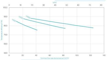
\*Test conditions following DIN EN 308:1997-06 (intake air: temp. 5 °C, humidity 70 %; extracted air: temp. 25 °C, humidity 50 %).
