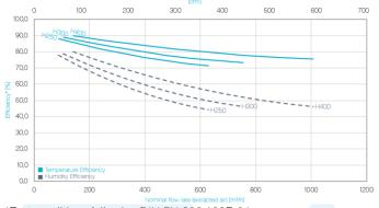
\*Test conditions following DIN EN 308:1997-06 (intake air: temp. 5 °C, humidity 70 %; extracted air: temp. 25 °C, humidity 50 %).
