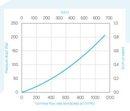
\*Based on a CORE height of 450 mm, test conditions following DIN EN 308:1997-06 (intake air: temp. 5 °C, humidity 70 %; extracted air: 25 °C, humidity 50 %)
