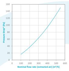
\*Based on a CORE height of 500 mm, test conditions following DIN EN 308:1997-06 (intake air: temp. 5 °C, humidity 70 %; extracted air: 25 °C, humidity 50 %)
