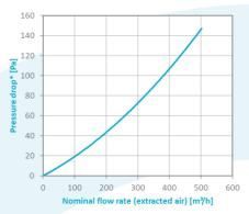
\*Based on a CORE height of 500 mm, test conditions following DIN EN 308:1997-06 (intake air: temp. 5 °C, humidity 70 %; extracted air: 25 °C, humidity 50 %)
