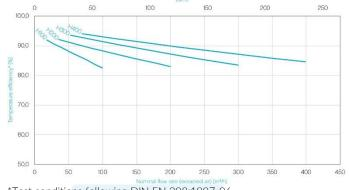
\*Test conditions following DIN EN 308:1997-06 (intake air: temp. 5  $^{\circ}$ C, humidity 70 %; extracted air: temp. 25  $^{\circ}$ C, humidity 50 %).
