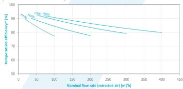
\*Test conditions following DIN EN 308:1997-06 (intake air: temp. 5 °C, humidity 70 %; extracted air: temp. 25 °C, humidity 50 %).
