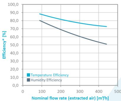
\*Based on a CORE height of 500 mm, test conditions following DIN EN 308:1997-06 (intake air: temp. 5 °C, humidity 70 %; extracted air: 25 °C, humidity 50 %)
