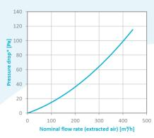
\*Based on a CORE height of 500 mm, test conditions following DIN EN 308:1997-06 (intake air: temp. 5 °C, humidity 70 %; extracted air: 25 °C, humidity 50 %)
