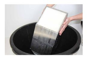
5. Empty the vessel and make sure none of the disinfectant remains in it. Put the Exchanger back into the vessel and thoroughly rinse it from all sides with clear water.
