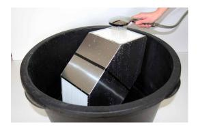
6. Pour a mild soap solution into all open sides of the Exchanger.
