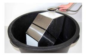
3. Spray every opening of the Exchanger (every open side) generously with the disinfectant to ensure a complete wetting of the membrane. Leave to stand for a couple of minutes.
