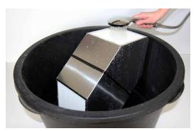
3. Fill the bottom of the vessel with a mild soap solution. Use a cup or similar to scoop the solution and let it flow into each opening of the Exchanger (every open side).
