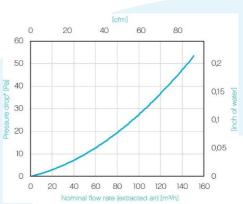
\*Based on a CORE height of 300 mm, test conditions following DIN EN 308:1997-06 (intake air: temp. 5 °C, humidity 70 %; extracted air: 25 °C, humidity 50 %)
