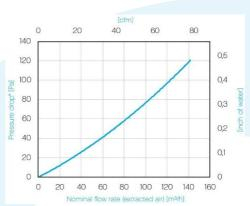
\*Based on a CORE height of 300 mm, test conditions following DIN EN 308:1997-06 (intake air: temp. 5 °C, humidity 70 %; extracted air: 25 °C, humidity 50 %)
